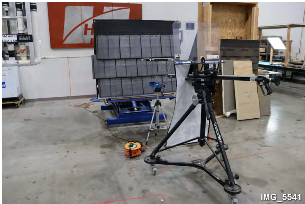
F5. Overview of test setup with Haag IBL-7 ice ball launcher.
