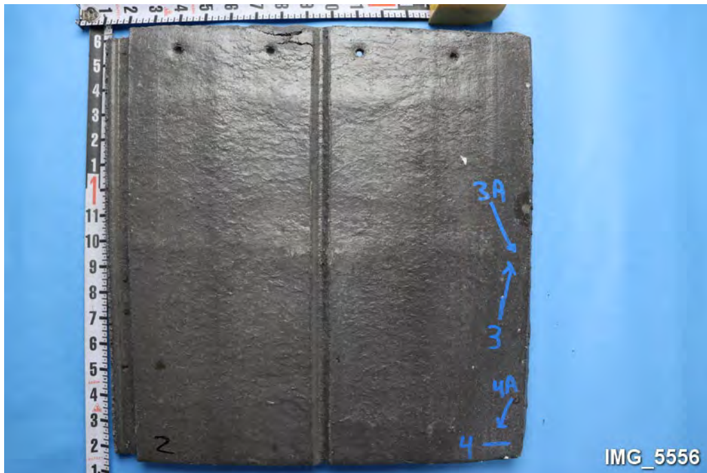
F13. Top of Tile 1 after impact testing. (Note 4 impact locations marked with paint.)
