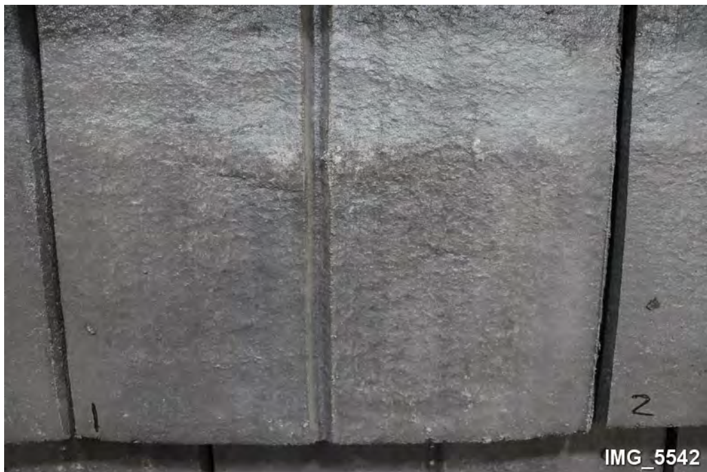
F8. Top of Tile 1 before impact testing.
