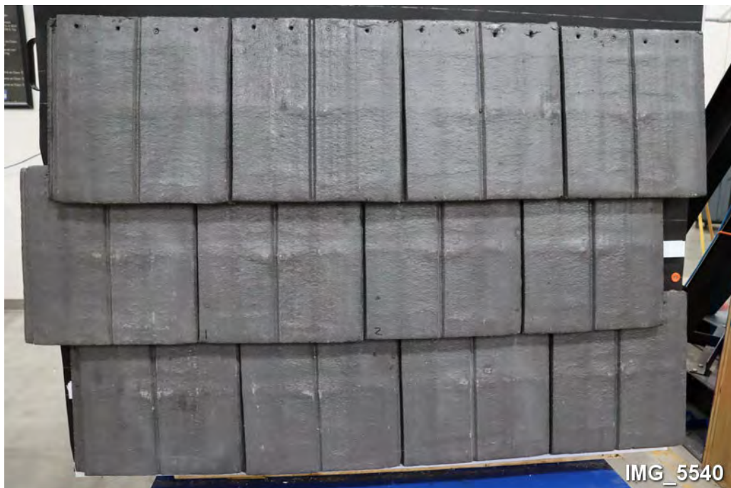
F6. Overview of test panel before impact testing.
