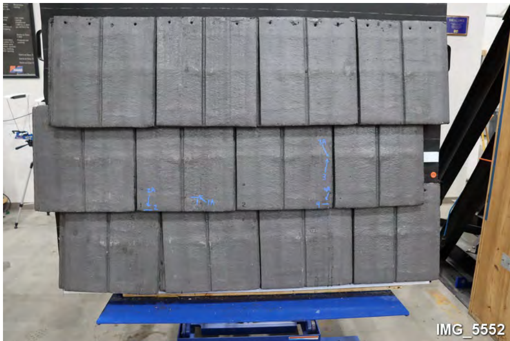
F7. Overview of test panel after impact testing.
