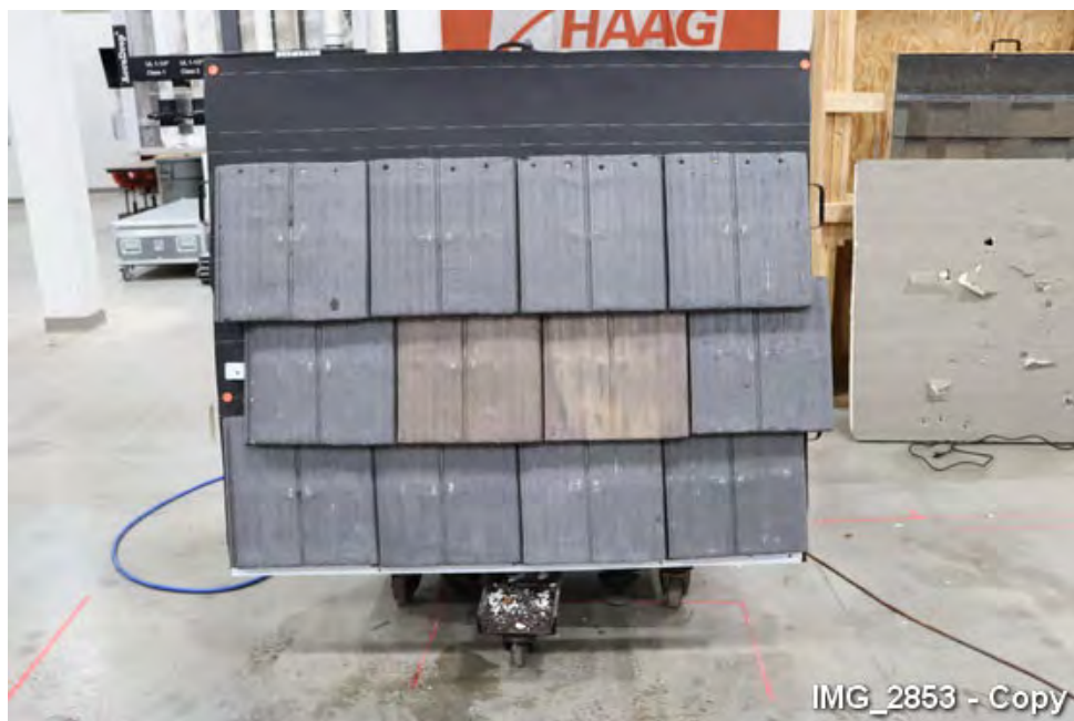
I6. Overview of test panel before impact testing.
