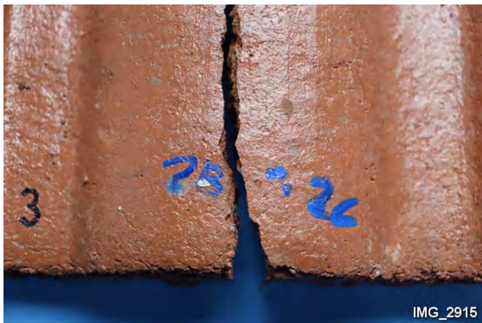
G20. Close-up of Impacts 2B and 2C. (Note tile did not break due to Impacts 2B and 2C.)
