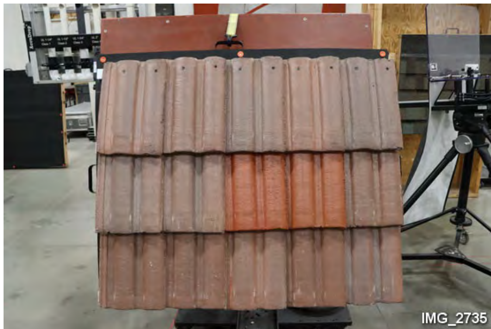
G12. Overview of test panel before impact testing.
