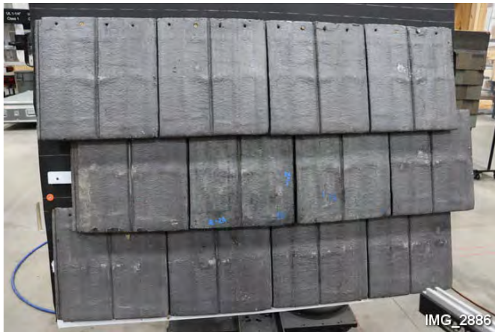
H7. Overview of test panel after impact testing.
