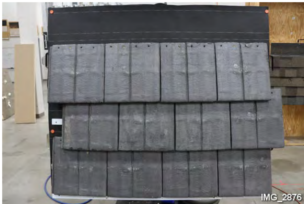
H14. Overview of test panel before impact testing.
