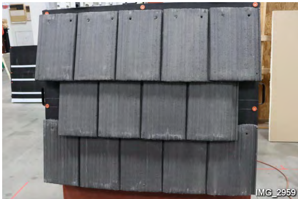
K12. Overview of test panel before impact testing.
