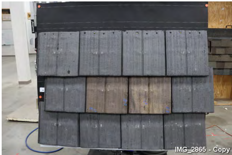
I13. Overview of test panel after impact testing.
