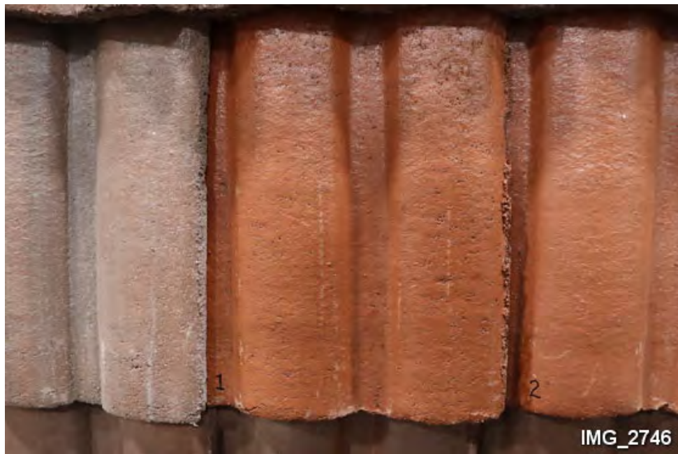
G7. Top of Tile 1 before impact testing.
