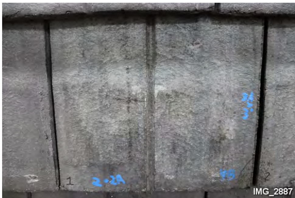
H8. Top of Tile 1 after impact testing. (Note 5 impact locations marked with paint.)
