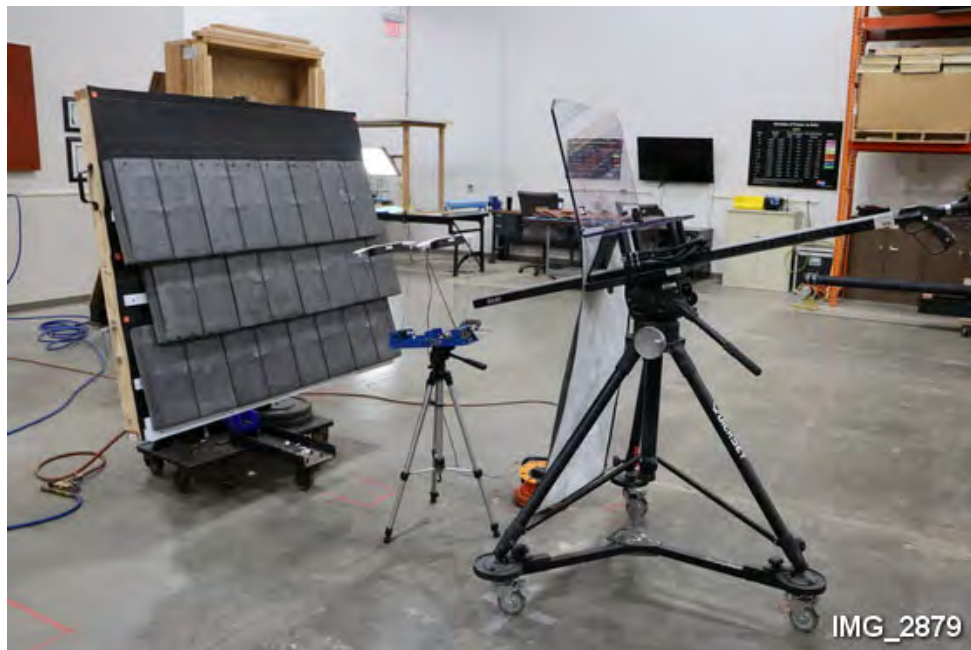
H5. Overview of test setup with Haag IBL-7 ice ball launcher.
