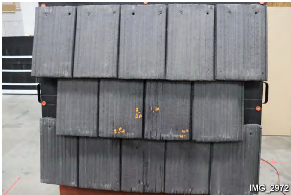
K13. Overview of test panel after impact testing.
