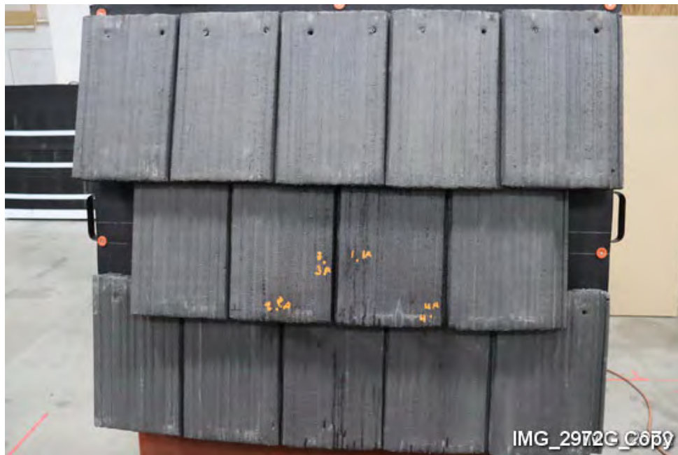
K7. Overview of test panel after impact testing.
