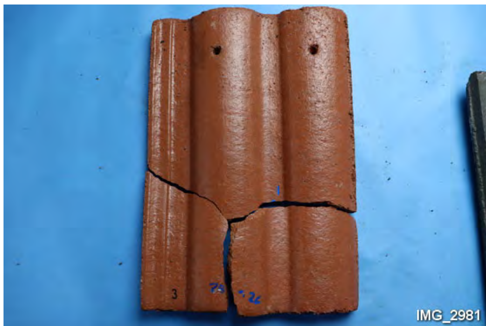
G18. Top of Tile 3 after impact testing. (Note tile broke at Impact 1 after not breaking at Impacts 2B and 2C.)
