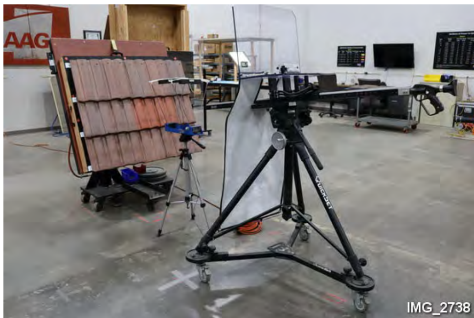
G6. Overview of test setup with Haag IBL-7 ice ball launcher.
