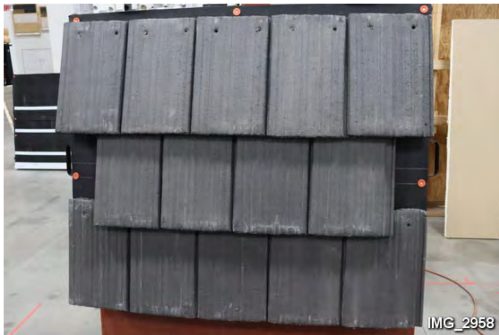
K6. Overview of test panel before impact testing.
