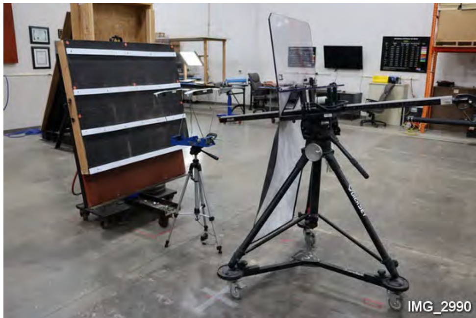
K5. Overview of test setup with Haag IBL-7 ice ball launcher.
