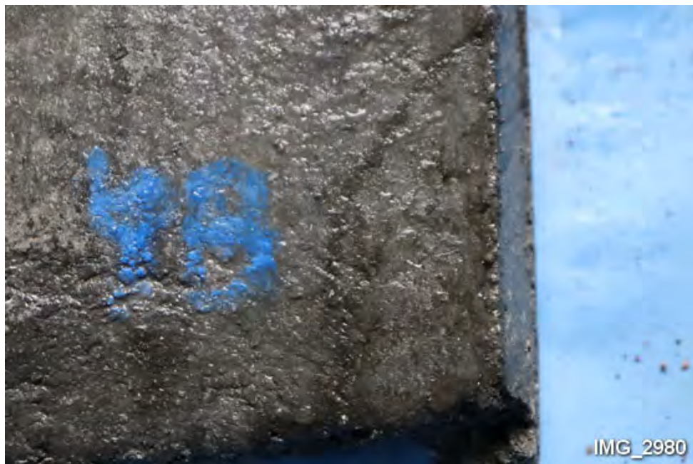
H12. Close-up of Impact 4B after wetting. (Note hairline crack.)
