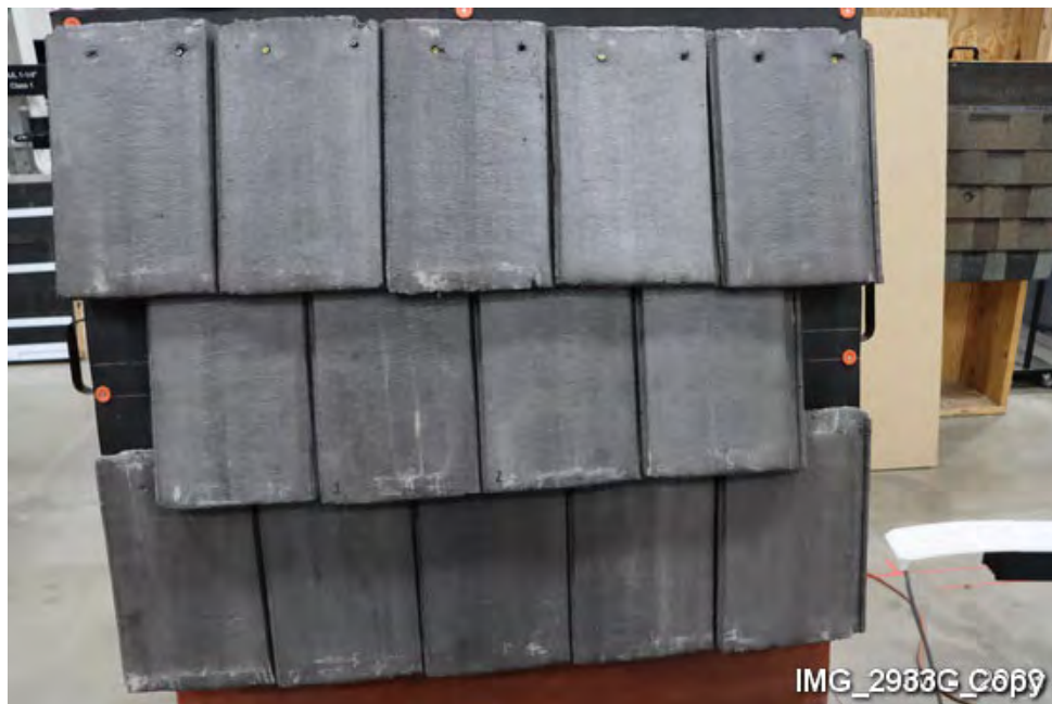
J12. Overview of test panel before impact testing.
