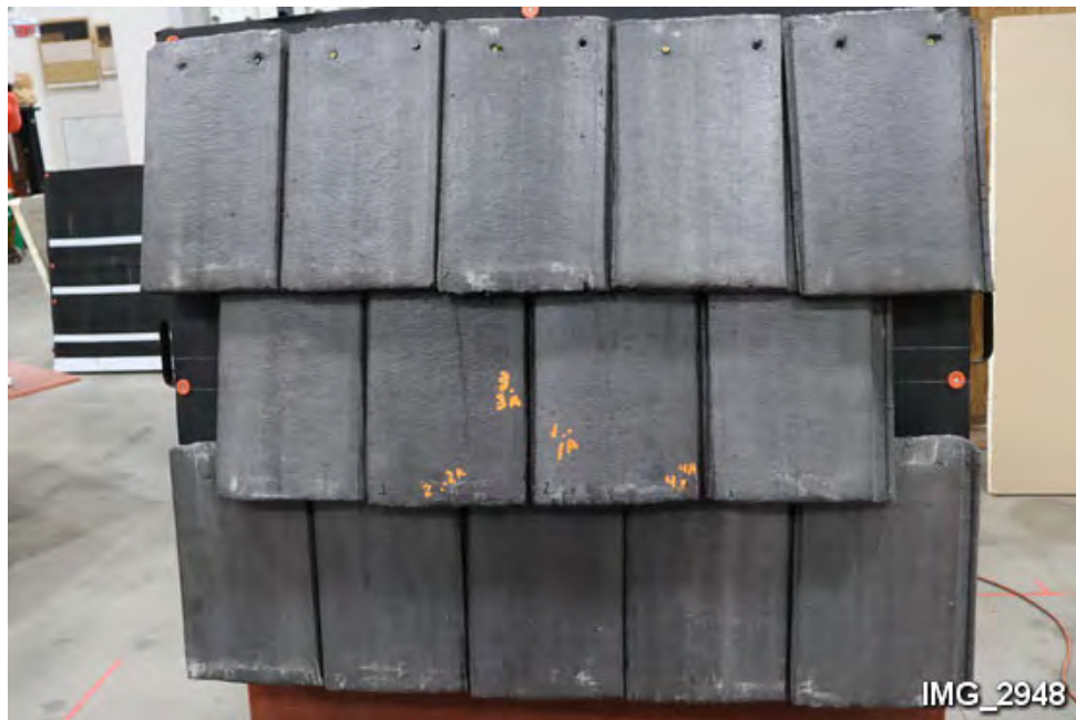
J13. Overview of test panel after impact testing.
