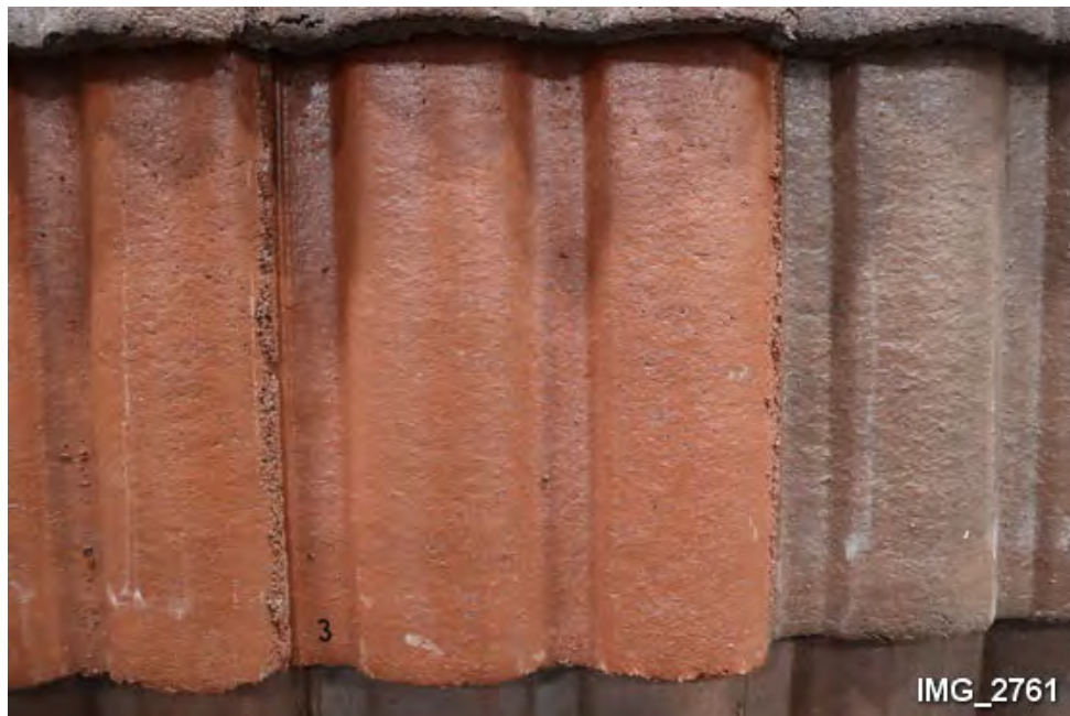
G17. Top of Tile 3 before impact testing.
