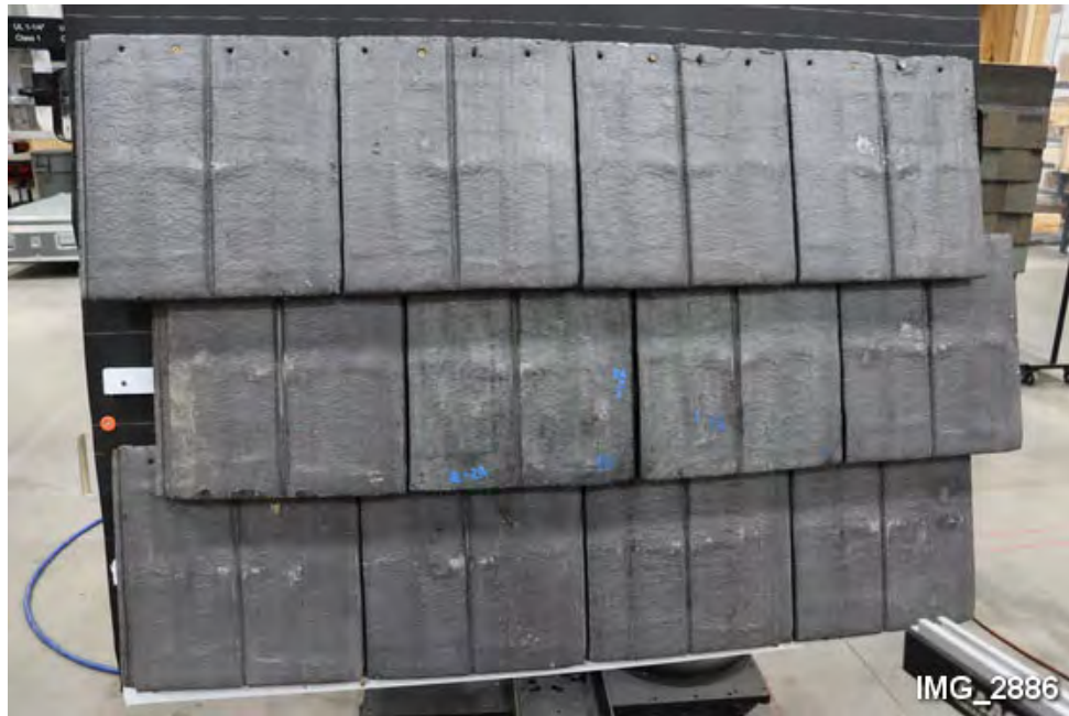
H15. Overview of test panel after impact testing.
