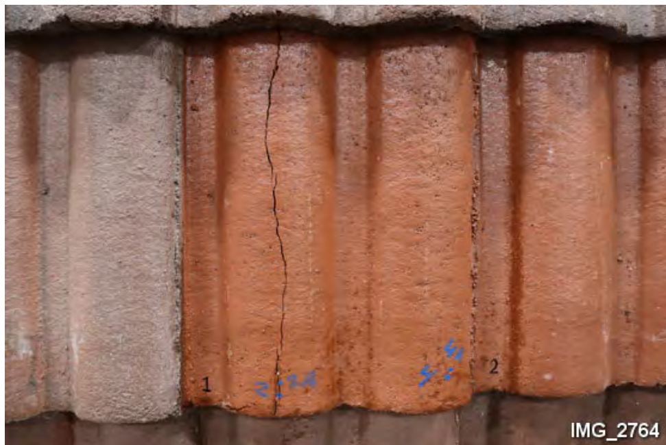
G8. Top of Tile 1 after impact testing. (Note four impact locations marked with paint.)
