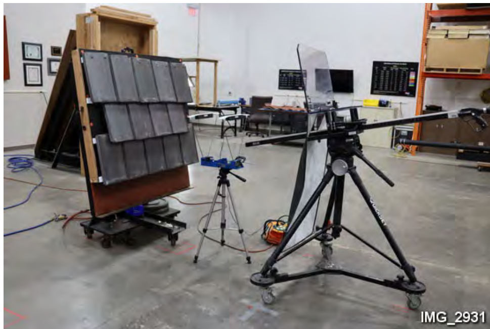
J5. Overview of test setup with Haag IBL-7 ice ball launcher.
