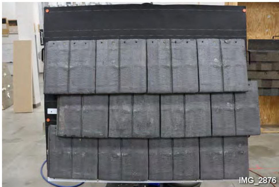
H6. Overview of test panel before impact testing.
