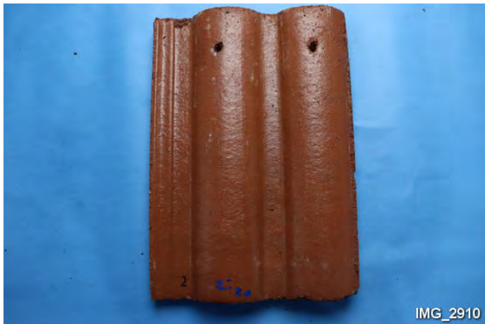
G14. Top of Tile 2 after impact testing. (Note 2 impact locations marked with paint.)
