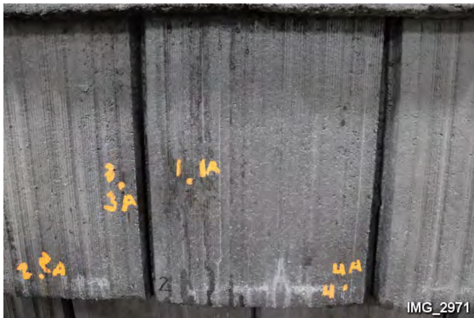
K14. Top of Tile 2 after impact testing. (Note 4 impact locations marked with paint.)
