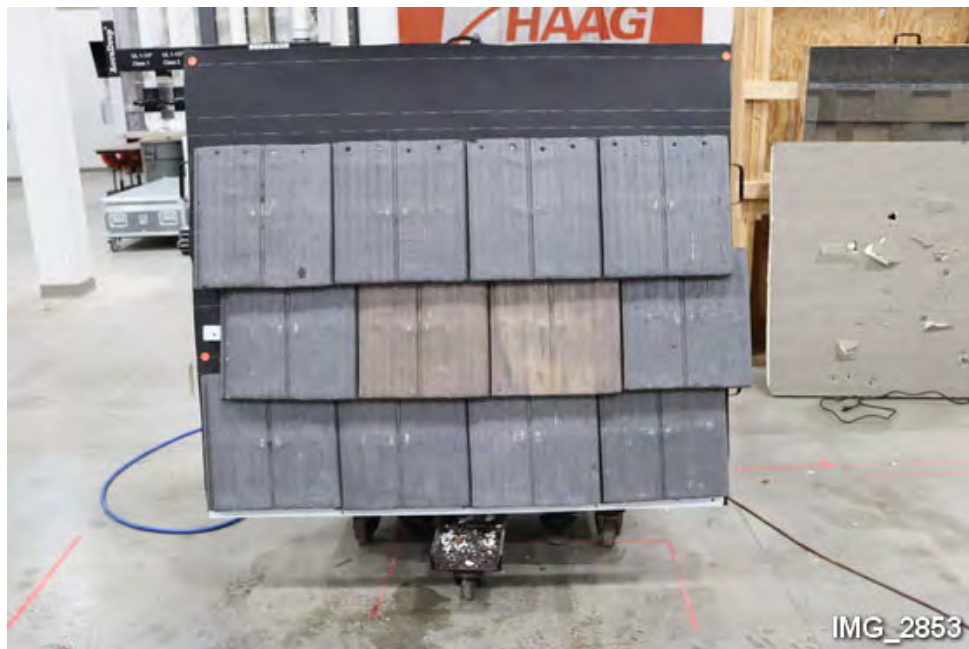
I12. Overview of test panel before impact testing.
