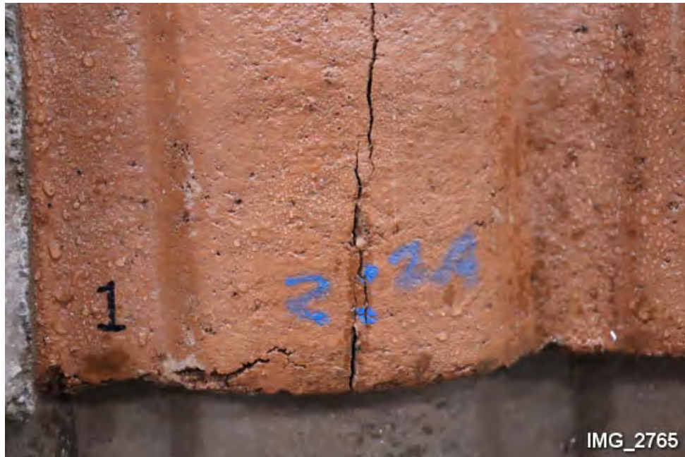
G9. Close-up of Impacts 2 and 2A. (Note tile broke with Impact 2A.)
