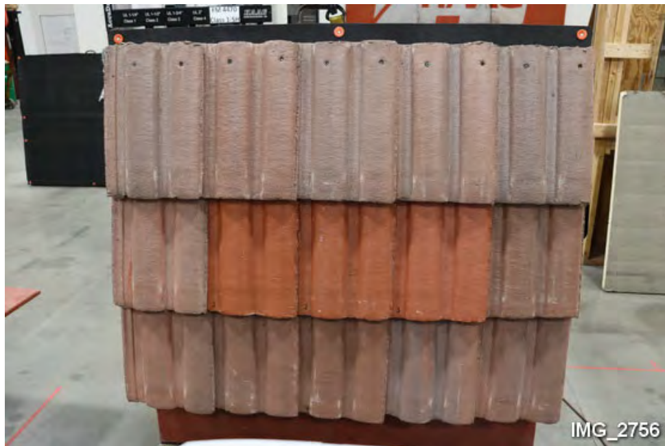
G5. Overview of test panel before impact testing.
