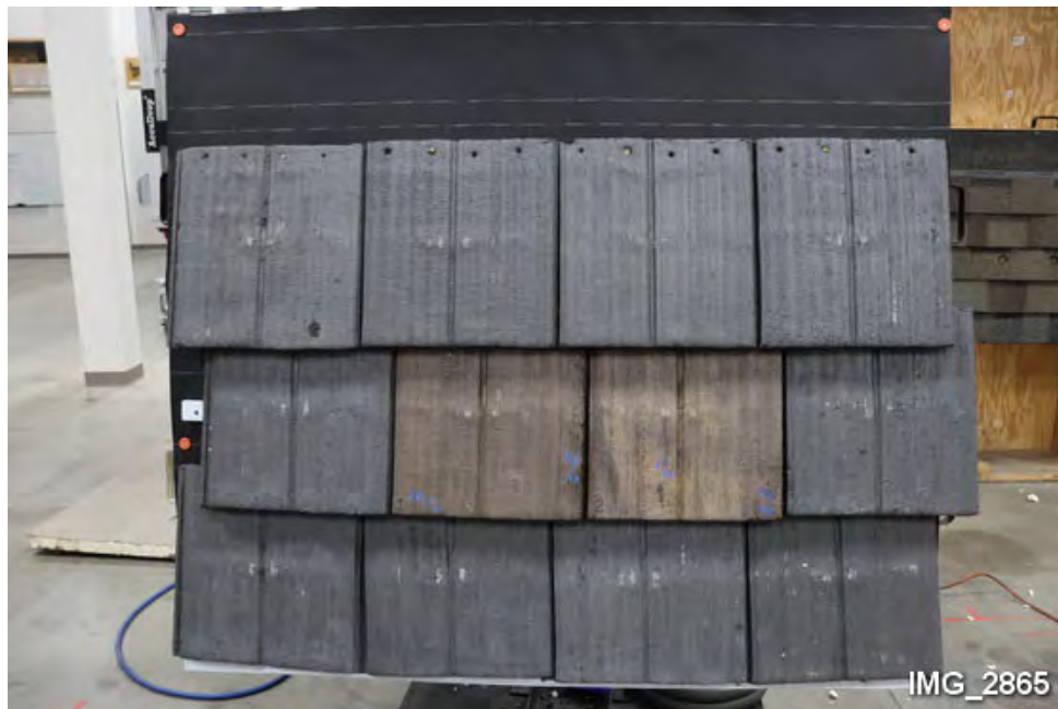
I7. Overview of test panel after impact testing.
