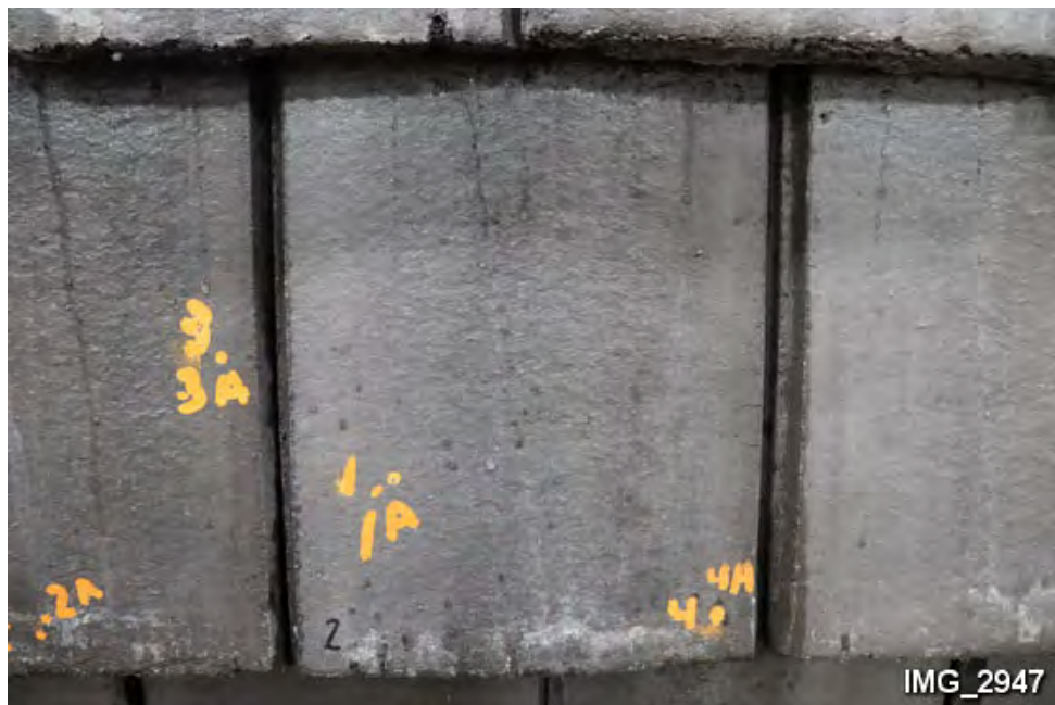
J14. Top of Tile 2 after impact testing. (Note four impact locations marked with paint.)
