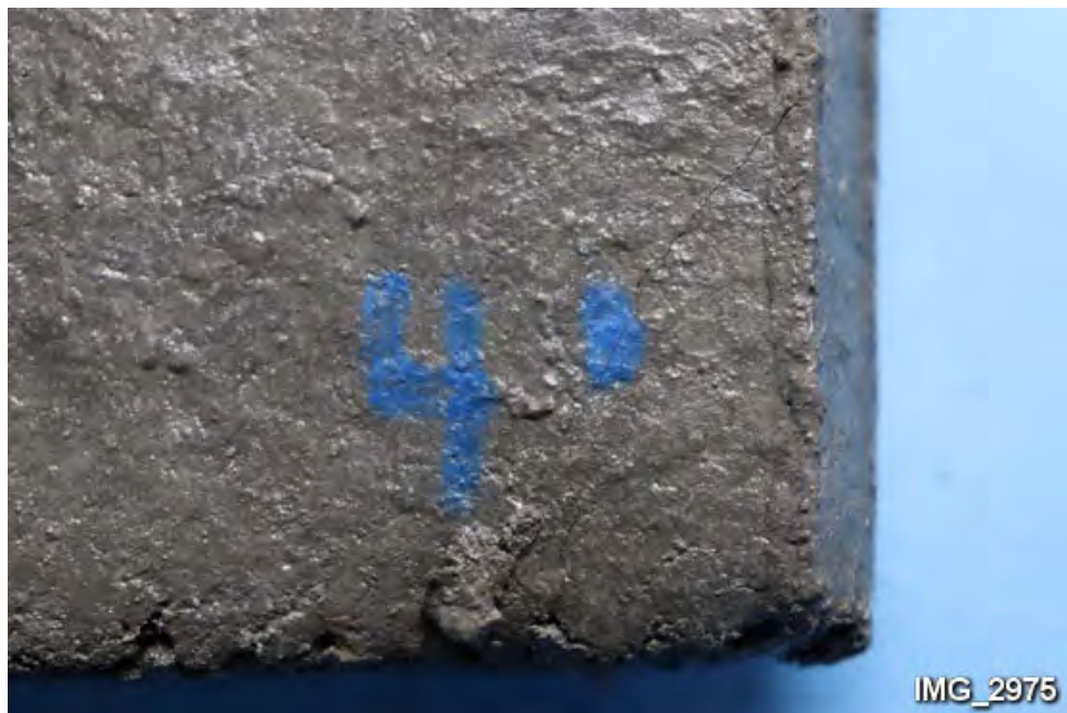
H18. Close-up of Impact 4. (Note hairline crack.)
