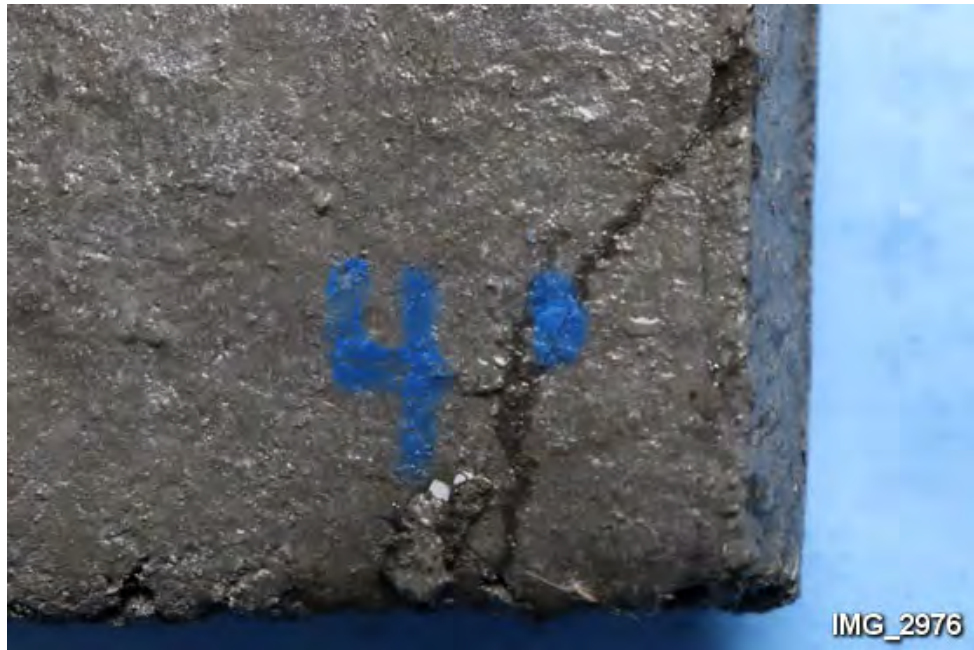
H19. Close-up of Impact 4 after wetting. (Note hairline crack.)
