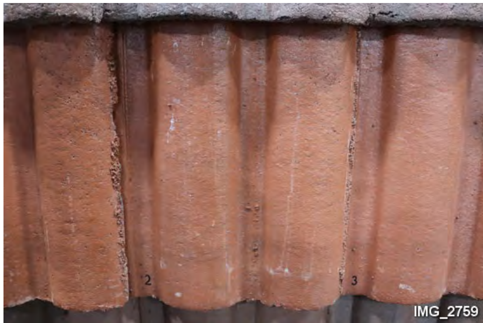
G13. Top of Tile 2 before impact testing.
