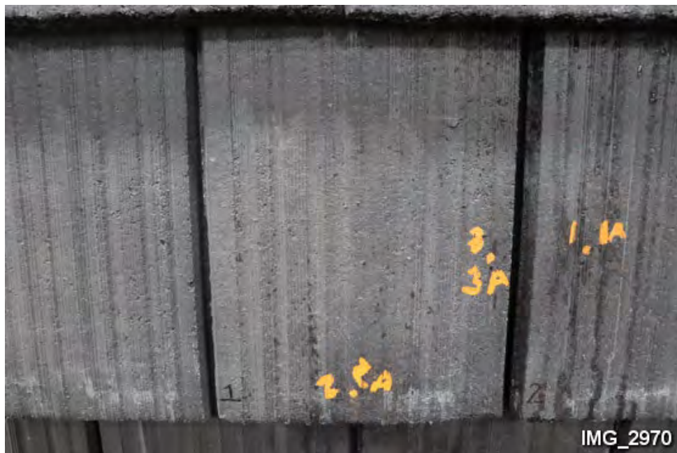
K8. Top of Tile 1 after impact testing. (Note 4 impact locations marked with paint.)
