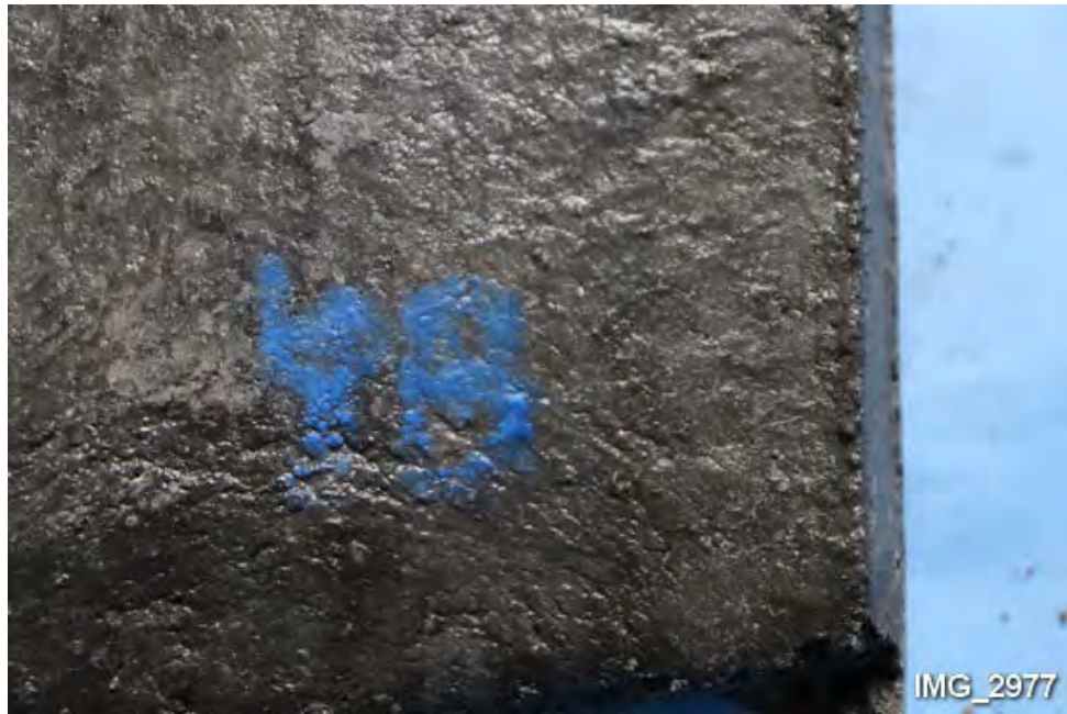
H11. Close-up of Impact 4B. (Note hairline crack.)
