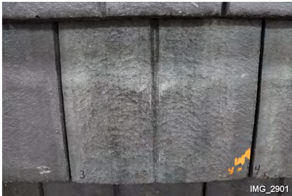
H23. Top of Tile 3 after impact testing. (Note 2 impact locations marked with paint.)
