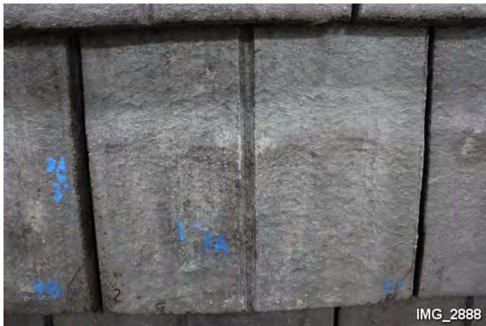
H16. Top of Tile 2 after impact testing. (Note 3 impact locations marked with paint.)
