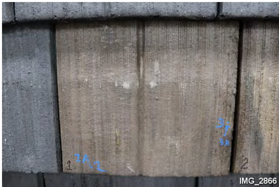
I8. Top of Tile 1 after impact testing. (Note four impact locations marked with paint.)
