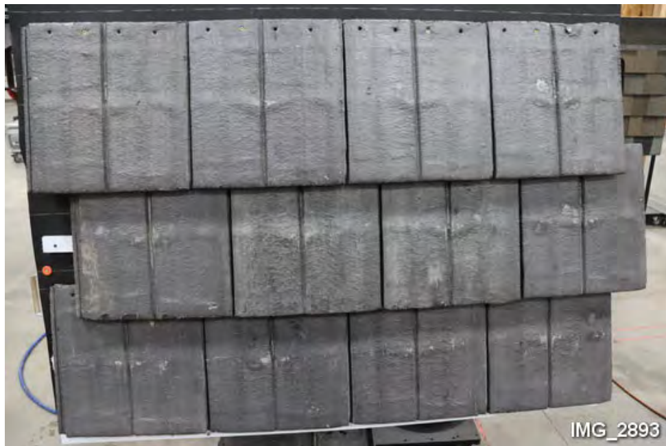
H21. Overview of test panel before impact testing.
