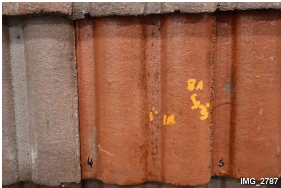
G23. Top of Tile 4 after impact testing. (Note 4 impact locations marked with paint.)
