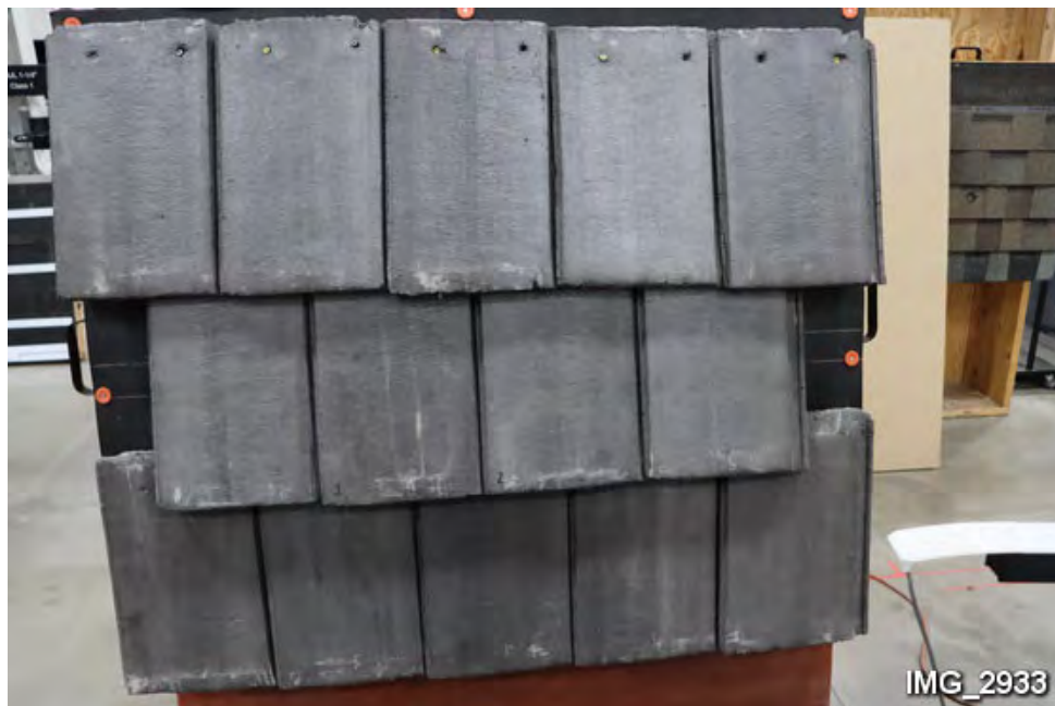
J6. Overview of test panel before impact testing.
