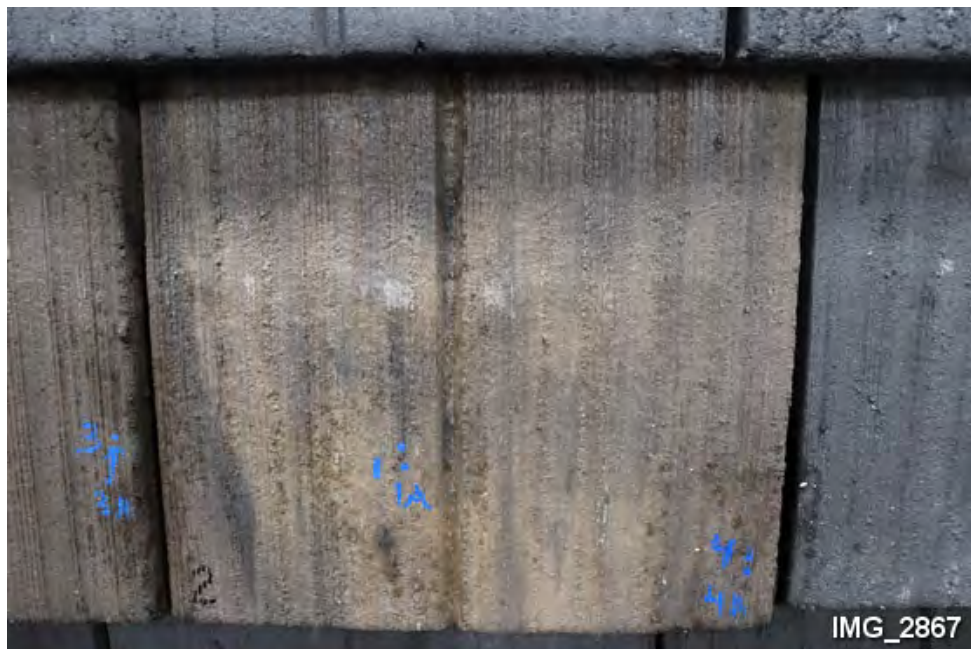
I14. Top of Tile 2 after impact testing. (Note four impact locations marked with paint.)
