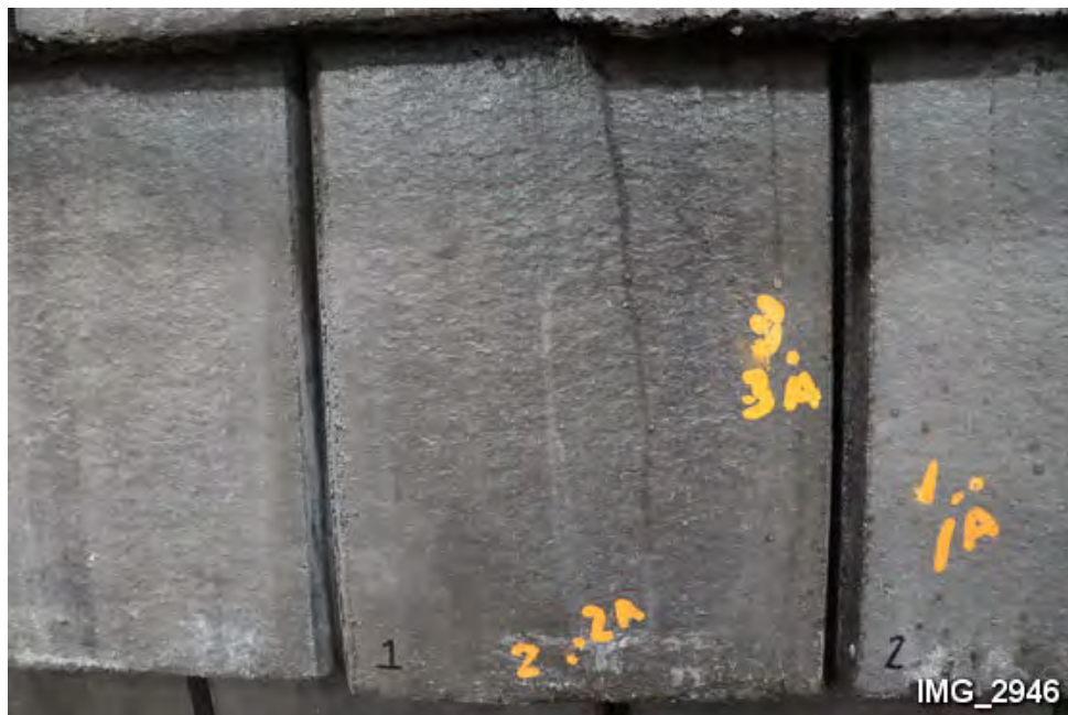
J8. Top of Tile 1 after impact testing. (Note four impact locations marked with paint.)
