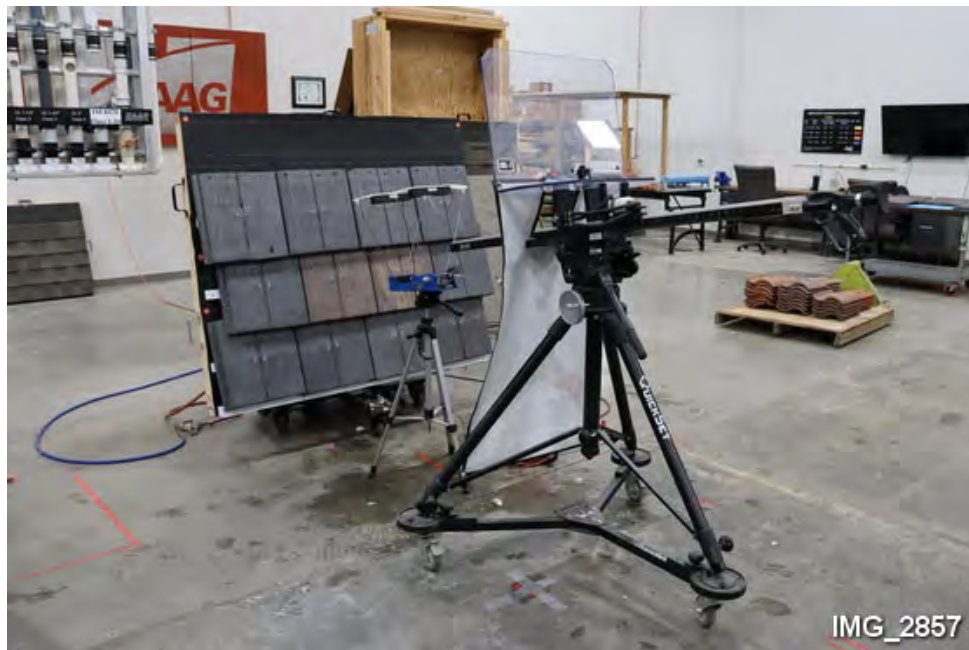
I5. Overview of test setup with Haag IBL-7 ice ball launcher.
