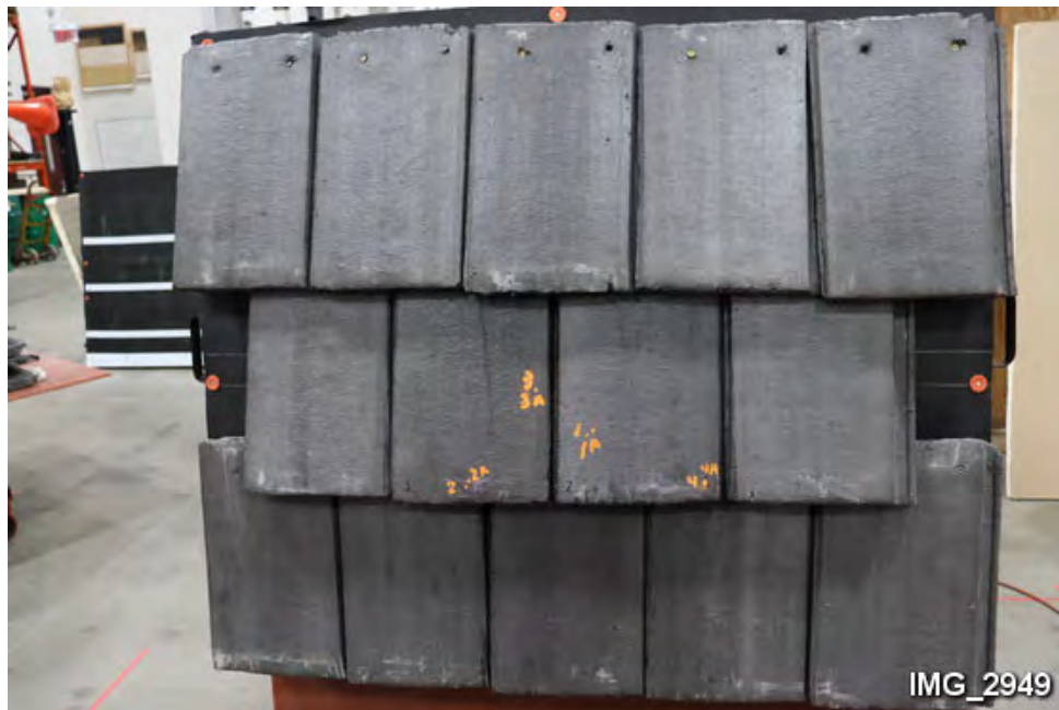
J7. Overview of test panel after impact testing.
